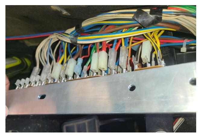
Load (right) side of the panel. Note the proximity of the connections. If you have bent any of the terminals, such that they are very close to each other, straighten them now. As you move the panel for attachment to the kick panel, wires may be pulled, causing terminals to touch.
