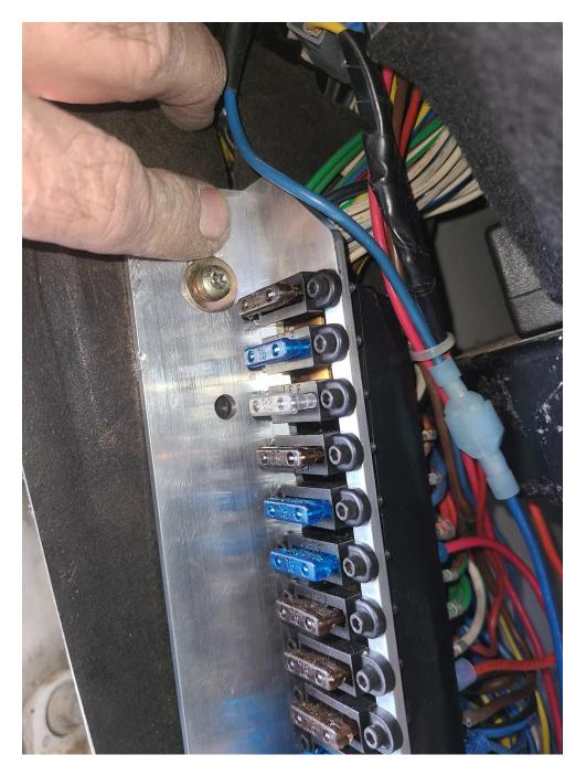
Now is the time to do any housekeeping. Replace and/or add any cable ties necessary, to keep your harness neat and tidy. More importantly, you want to bundle the harness as close to the back of the fuse panel as possible. On later cars, SRS vehicles with the knee bolster, the bracket will complicate things at the top. You will need to work the harness so it clears. Don't worry, plenty of room in the area above the panel.
