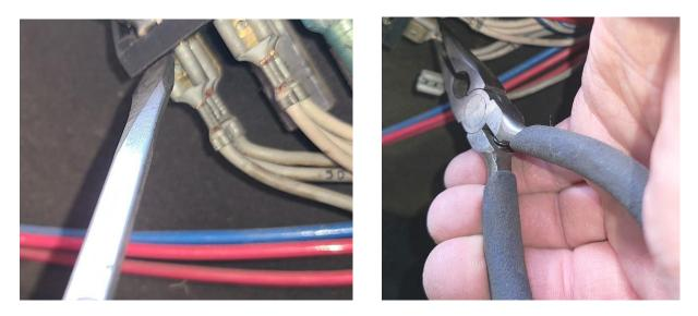
If any of your old connectors, from the car's harness, are loose, now is the time to crimp them shut, so that they grab your new panel's terminals tightly. Don't CRUSH them! Too tight, and you will not be able to install them. Examine each one carefully for cracks. If you find one loose, and it will not tighten down, there is a good chance it is cracked. Cut it off and replace it before continuing.
