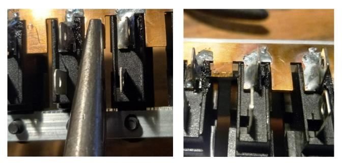
With the buss's tab raised, you can slip a standard, ¼" female spade terminal onto the tab. Wire that connector to the supply side of the desired accessory fuse holder. Remember to check for proper wire gauge for the amperage you plan to run in that fuse holder. Shown is a 14-16 gauge terminal.
